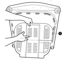
3 Insert the 2 screws 2 into the holes to assemble the anti-rat cover to the appliance.
